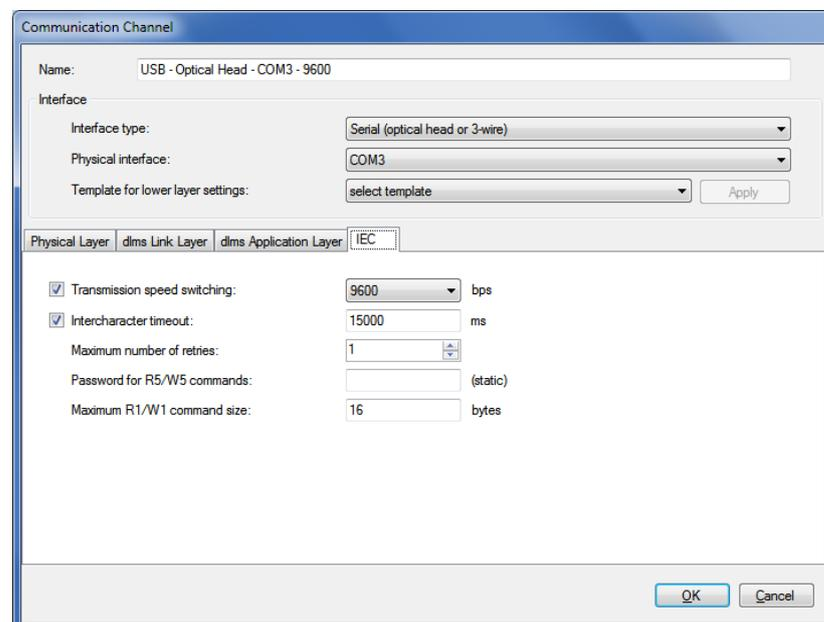
2. Select the required maximum transmission rate (default = 9600 bps) in the "Transmission speed switching" drop down list. Untick the checkbox if you don't want to allow transmission rate switching.
