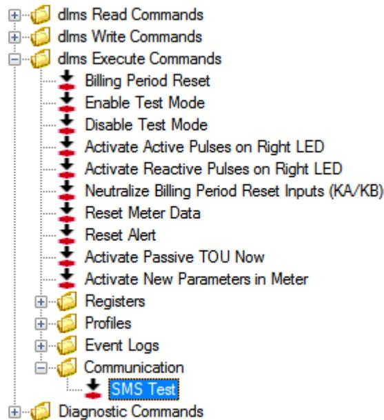
The "SMS Test" dialogue window appears. In this window you can enter the phone number to be called and the message text of the test SMS.
