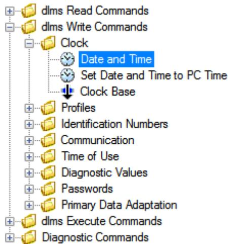
With write commands, the current parameter or value is always read out first from the device and displayed in a dialogue window for modification, e.g. for setting time and date:
