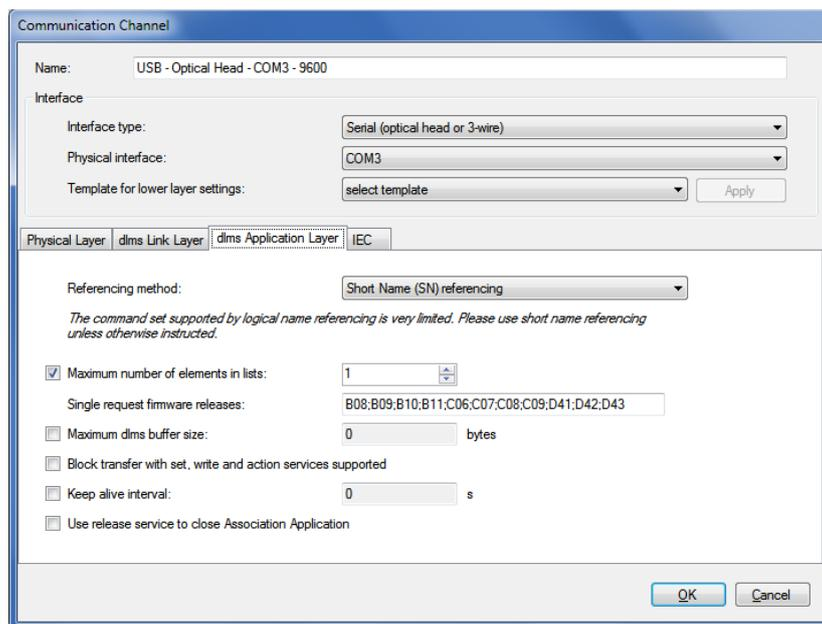
2. Select "Short name (SN) referencing" or "Logical name (LN) referencing" method. The command set supported by LN referencing is very limited. The .MAP tools only work with short names. Therefore SN referencing is the preferred choice unless otherwise instructed.
