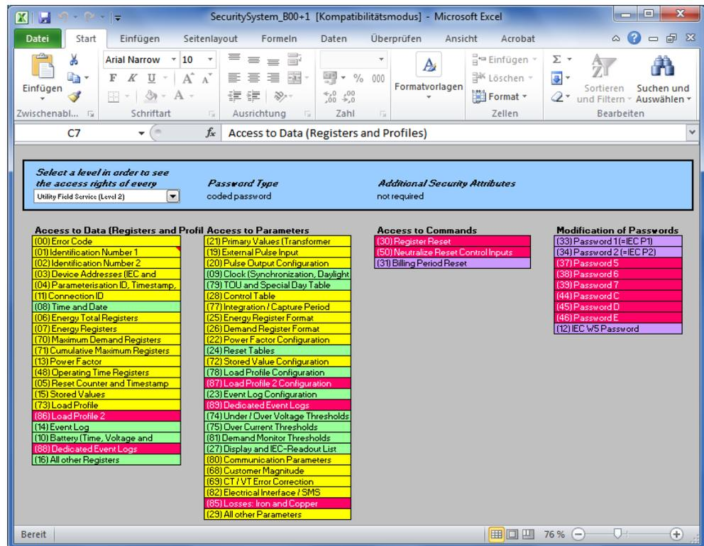
The desired security level can be selected in the drop down list at top left. The access rights for the level selected for individual data, parameters, commands and passwords are then displayed by means of colours according to the colour code.
