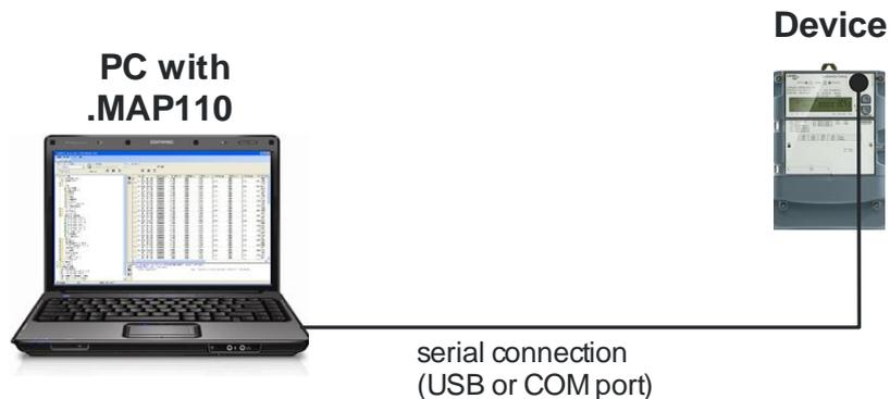
A device ready for operation and an optical reading head for connection to a serial interface (USB or COM port) are required for this purpose. The Landis+Gyr .MAP110 Service Tool must also be installed on the PC and licensed, e.g. for user group "Installation".
