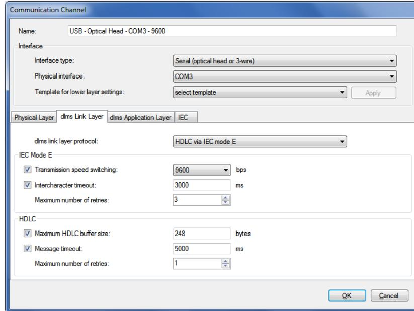
2. Select the required protocol for the planned activity in the "dlms Link layer protocol" drop down list. Possible settings:
