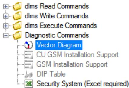
A vector diagram is shown in the "Vector Diagram" window, which is calculated from the continuously read instantaneous values of voltages, currents and phase angles. The individual instantaneous values measured by the meter are displayed next to the diagram.
