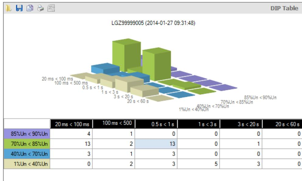
The categories, i.e. the severity of the voltage failures, are shown in colour, e.g. voltage failures of 1 to 40 % of rated voltage in violet. The table contains a line for each category, the diagram a series of bars in the x-direction.
