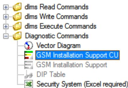
The field strengths of the cell logged in and all neighbouring cells are displayed in the "GSM Installation Support" window. When used on the spot this allows the optimum antenna position to be determined or a check of the received field strength.
