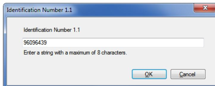
Modify the data displayed and then click on **Ok**. The modified data is written in the device and recorded in the command log window (command left, value right):
