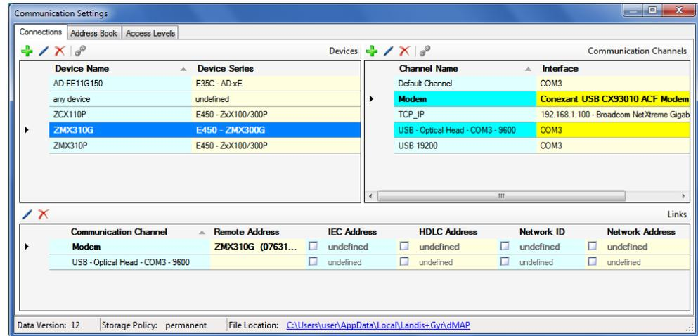
In the figure below a communication channel is selected in the "Communication Channels" area (highlighted blue). All the linked devices are also highlighted in the "Devices" area (light blue/yellow) and the links with their attributes are shown in the "Links" area.
