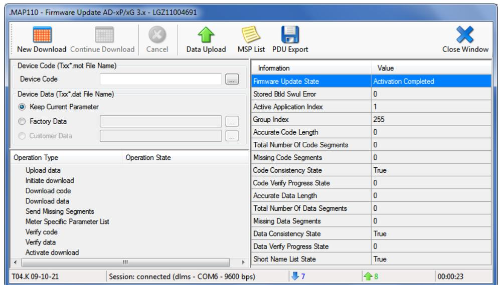
Enter the name of the MOT file with the new firmware release in the entry field "Device Code" or select a file in the "Select Device Code File" window, which appears after clicking on .
