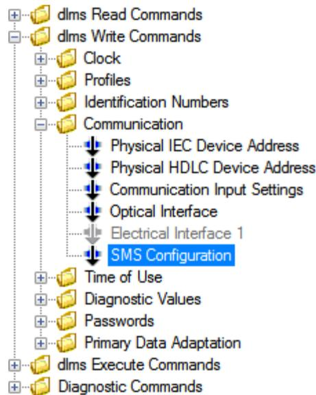
The SMS configuration data is displayed in the dialogue window. You can modify the phone number, the message text, the initialisation string and the transmission parameters.
