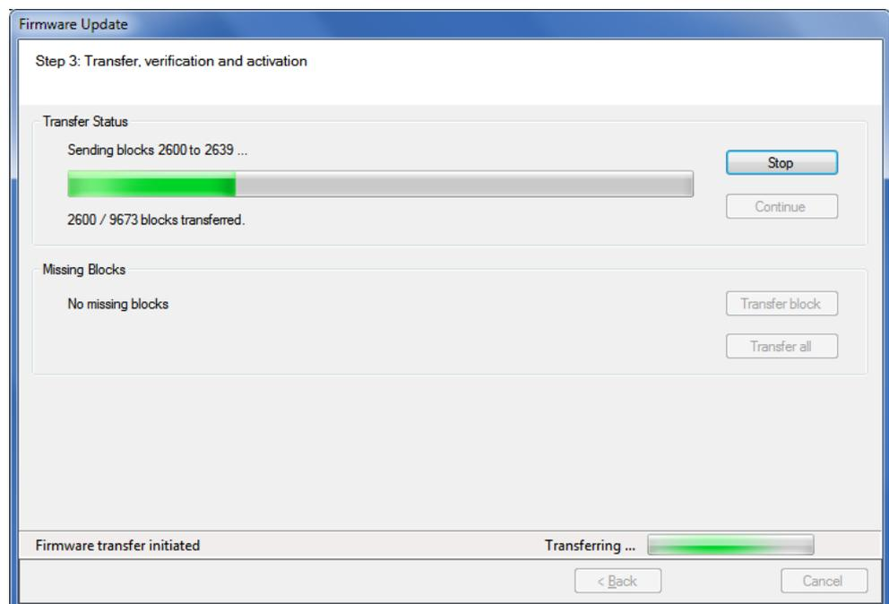
Wait until all blocks are transferred and verified and the subsequent firmware activation is started. Then the following display appears:
