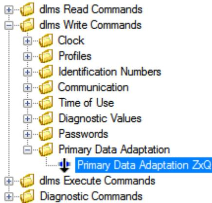
In the dialogue window you can modify the primary value adaptation settings of transformer connected devices.
