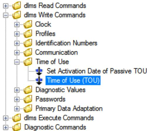
In the dialogue window "Time of use (TOU)" you can modify the TOU read out from the device and write it back again into the device. You can also save a read out TOU in a XML file or load a saved XML file into the .MAP110 to write it into the device.
