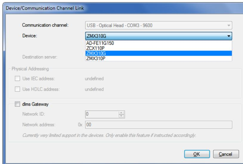
4. In the "Communication Channel" drop down list select one of the defined communication channels (or alternatively in the "Device" drop down list one of the defined devices).
