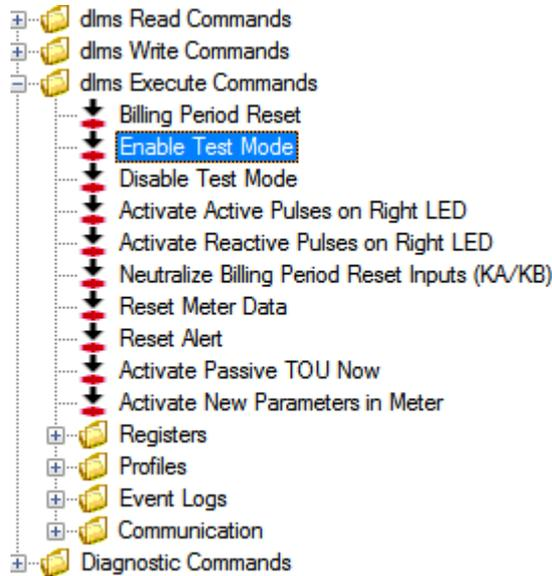
The execute command is normally transmitted to the device without additional dialogue (exception: see 7.3.1 "SMS test transmission") and executed there. The commands executed are recorded in the command log window:
